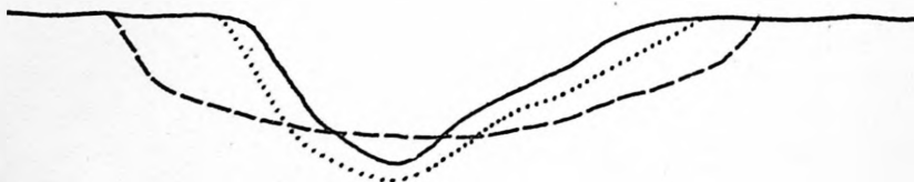
FIG. 7. Let the solid line represent the cross-section of an alluvial river in its natural state. If the discharge be increased the cross-section will be increased and it is generally assumed that the increase will be as indicated by the dotted line. The fact is, however, that the change will ordinarily result in a decrease in mean depth with corresponding increase in width as indicated by the broken line.
